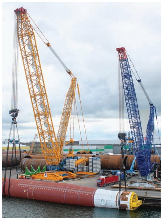
A 2,500-mt lift capacity crawler crane at Sarens' facility in Rostock, Germany. Sarens
